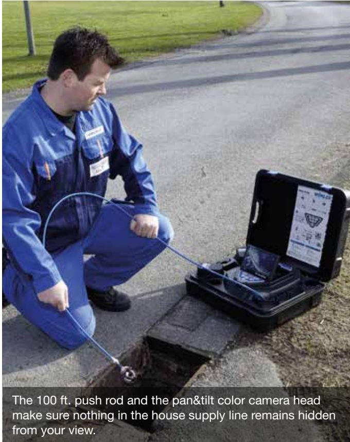
The Wohler VIS 350 precisely locates radio waves transmitted by the camera head through concrete and asphalt to save a lot of time and further building damage.
